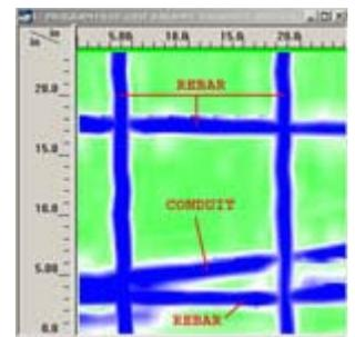
performed about 40 line scans over a 20-foot by 40-foot area with a Structure Scan to determine the location and depth of each section of tubing. He scanned the area, marking the location of any tubing in each area as he went. Then, he was able to map out the pattern of the tubing to let his clients know where it was safe to cut.
