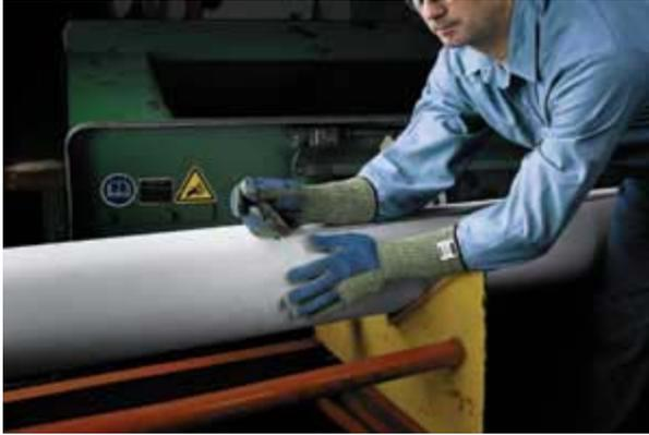
**SuperFabric®** combines multiple layers of specialty materials with varying thicknesses. Typical applications include metal forming and stamping.
