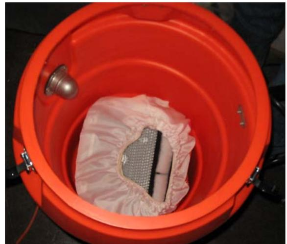
Figure 2. Vacuum debris holding container with fallen filter in the bottom. Notice the lack of double-sided tape on the black portion of the filter.
