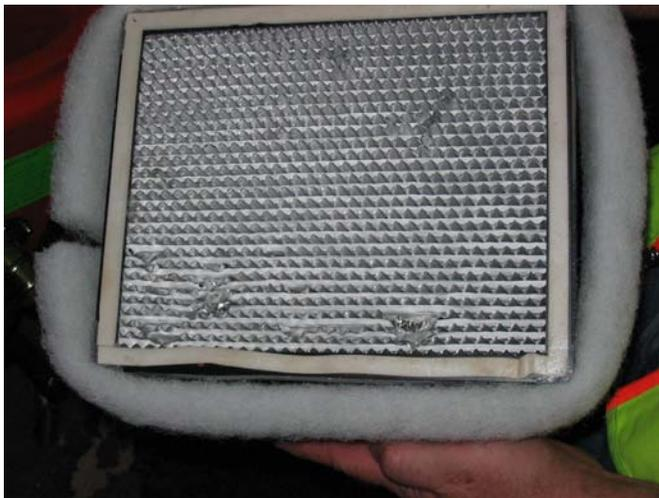
Figure 1. HEPA Filter. Notice the white tape around the edge and how it lifts at the bottom of the filter, showing that it is not very adhesive.
