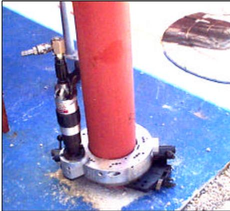
**Figure 4. Clamshell mounted at floor level.**
