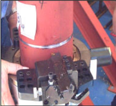
**Figure 6. Clamshell showing rotating mechanism with star wheels and cutting tip in place.**
