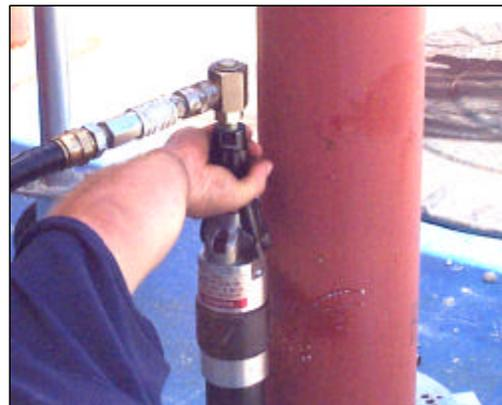
**Figure 5. Deviant wrist position caused by placement of the clamshell.**
