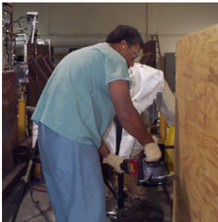
Figure 1: (Left) An operator making a horizontal cut in the plywood with the Adamant circular saw.
