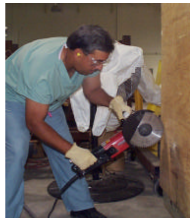
Figure 1: (Left) An operator making a horizontal cut in the plywood with the Adamant circular saw.
