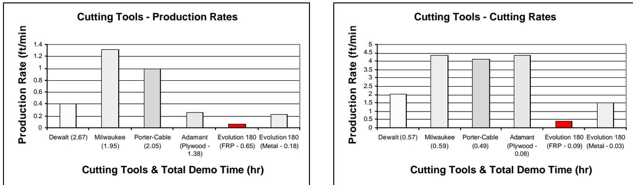
**NOTE:** Dewalt, Milwaukee, Porter-Cable, and Evolution 180 circular saws were tested on glovebox FRP crates. Adamant saw was tested on a plywood crate, and the Evolution 180 was also tested in metal.
