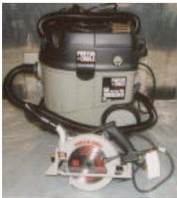
**Figure 1. Porter-Cable circular saw (743K) with vacuum system.**
