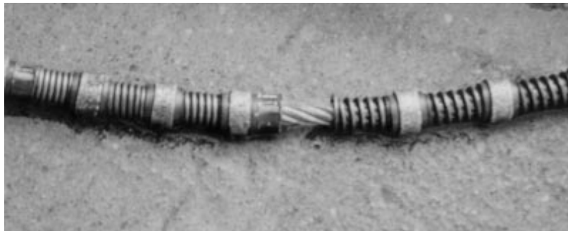
Figure C-3. Damaged wire from Perma-Fill cut.
