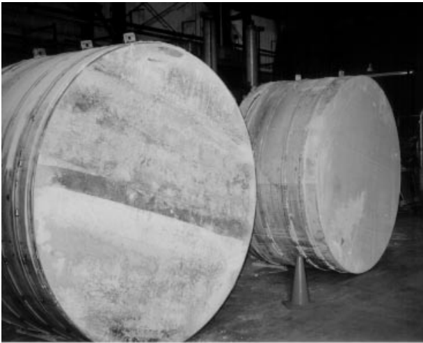
Figure C-1. Rheocell – 15 and Mortar Void Filled Mockups..
