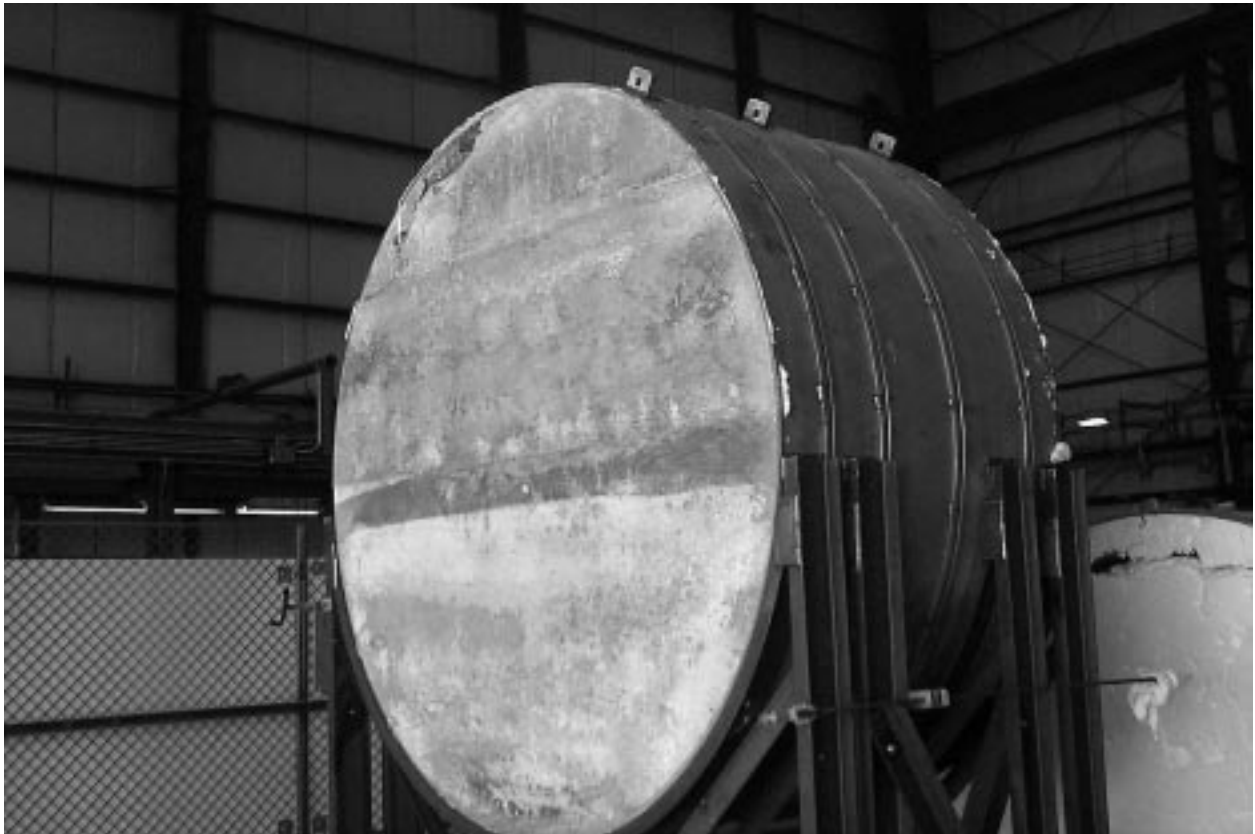
Figure 7 Picture of Vacuum Vessel Surrogate filled with Rheocell-15
