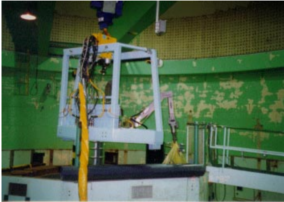
Figure 4. The DAWP Suspended from the Crane Removes Trash from the Reactor Top
