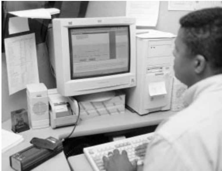
Figure 8. NITON® XL-800 Series Multi-Element Analyzer downloading results to a PC
