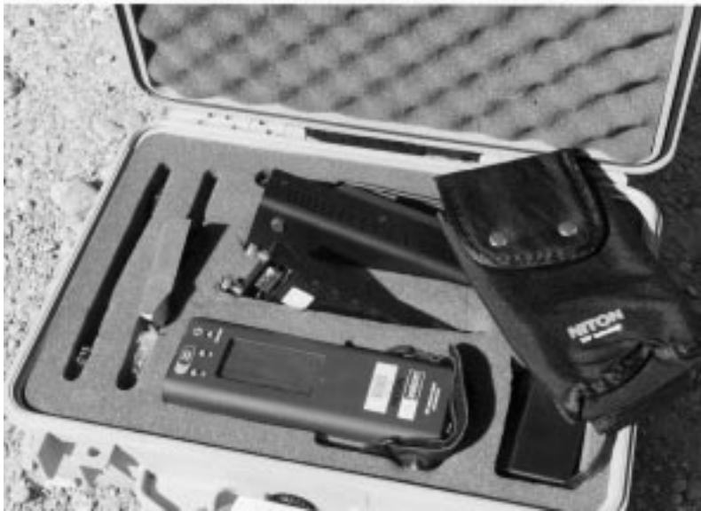
Figure 3. Basic NITON® XL-800 Series Multi-Element Analyzer system. Shown are the NITON® analyzer, spare battery and charger system, irregular shape adapter, computer connector cable, and the waterproof, hard-sided carrying case.
