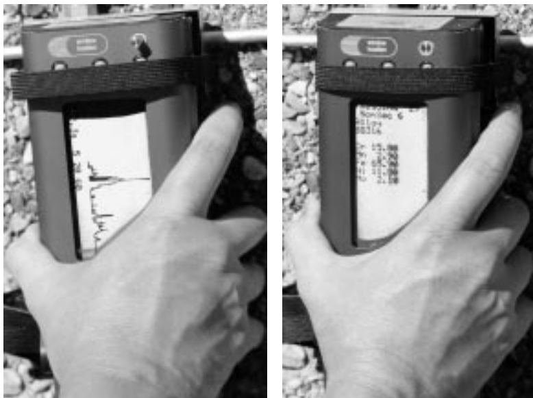
Figure 1. NITON XL-800® Series Multi-Element Analyzer analyzing a small metal part using the irregular shaped part adapter. The image on the left shows the energy spectrum the instrument is reading during the analysis process. The image on the right shows the final element concentrations and alloy determination.
