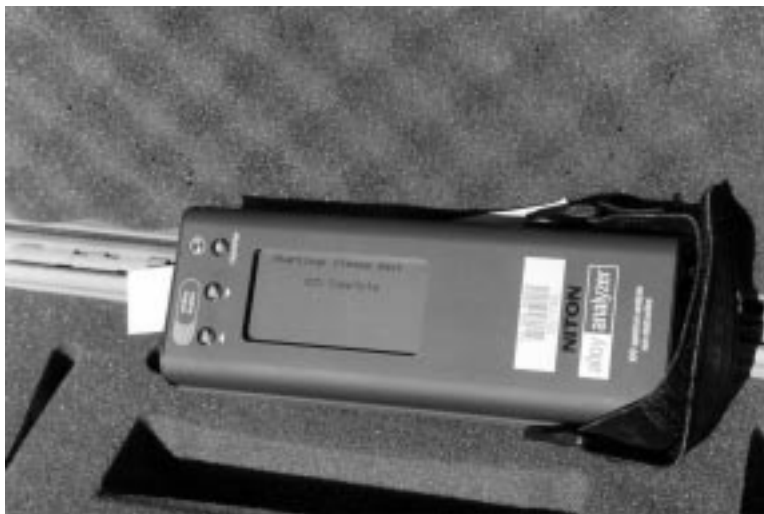
Figure 6. NITON® XL-800 Series Multi-Element Analyzer performing self-calibration
