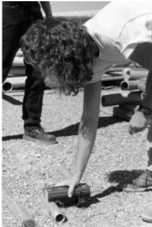
Figure 10. NITON® XL-800 Series Multi-Element Analyzer being used to identify and separate metal scrap
