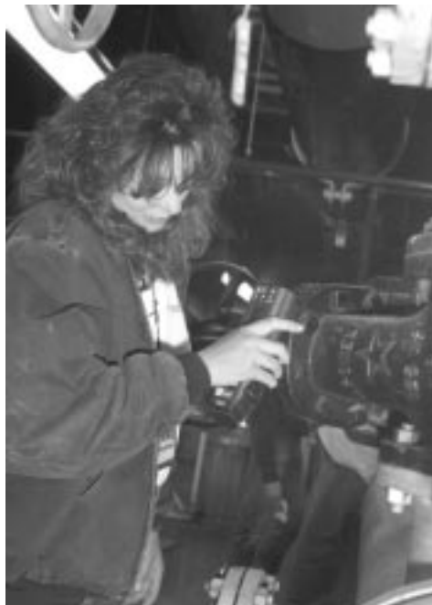
Figure 7. NITON® XL-800 Series Multi-Element Analyzer analyzing a system valve in place.
