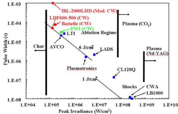
Figure 1. Range of peak irradiance vs pulse width for laser paint stripping trials over 25 years.
