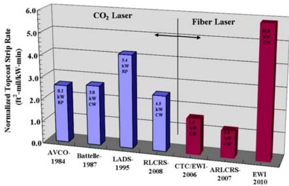
Figure 9. Normalized strip rates on typical aircraft paint
