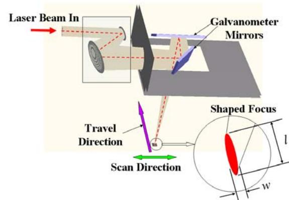
Figure 2. Typical galvo configuration for laser paint stripping.
