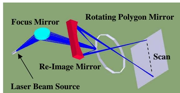
Figure 5. Fully reflective polygon scanner design
