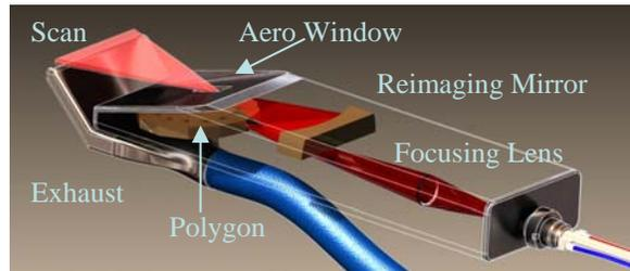
Figure 4. EWI patent-pending polygon scanner design
