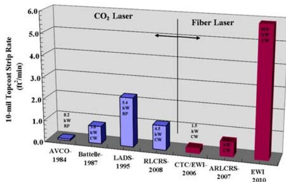
Figure 10. Laser paint stripping rates on typical aircraft paint
