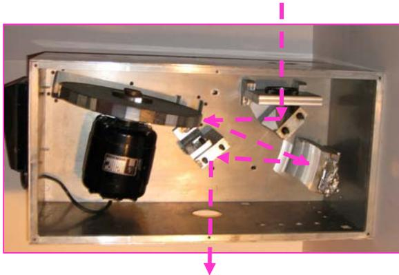
Figure 3. Early (1986) polygon scanner developed by Walters and Ream at Battelle
