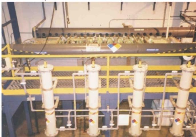
Figure 2. Top view of electrorefining cell.
