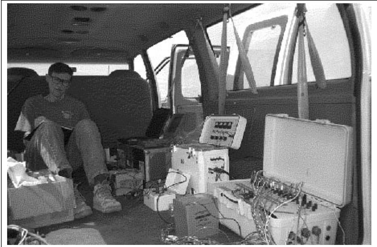
Figure 4. The field operations center for an Electrical Resistance Tomography For Subsurface Imaging network is typically located in a van or truck. A fast laptop computer can be programmed to process the data collected into two- or three-dimensional tomographs for site investigators to use on-site. Once the subsurface electrode arrays are emplaced and the network is set up, it can be run by a technician or put in automatic mode.
