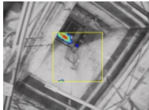
Figure 14 Image of Sources under Shield Cover
