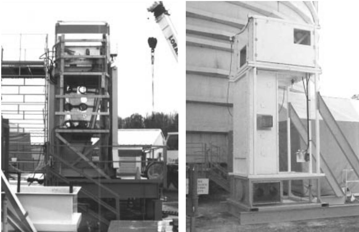
**Figure 21 The Houdini-II TMADS (picture do right) provided a sleeker design with more room for maintenance activities than the Houdini-I TMADS had provided (pictured on left).**
