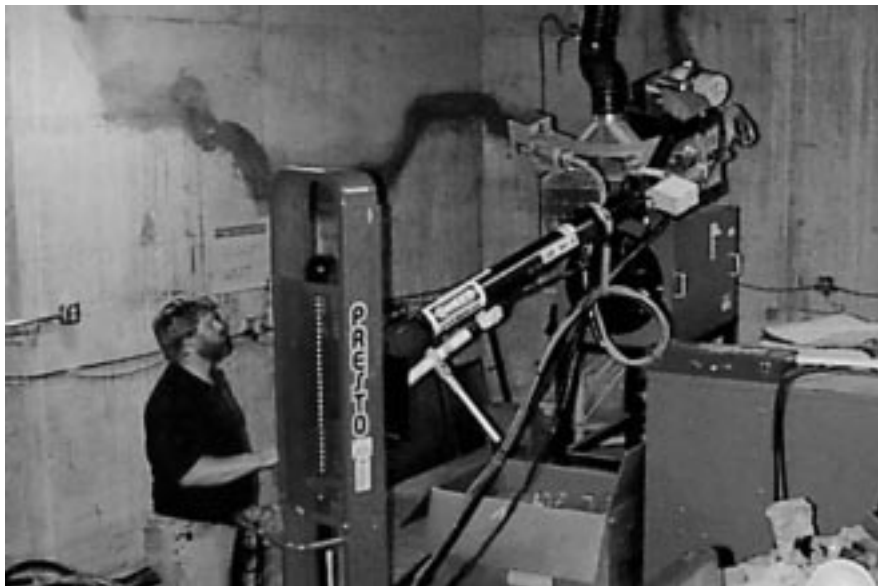
Figure 12. C-Frame Inspection Head at the End of Adjustable Boom
