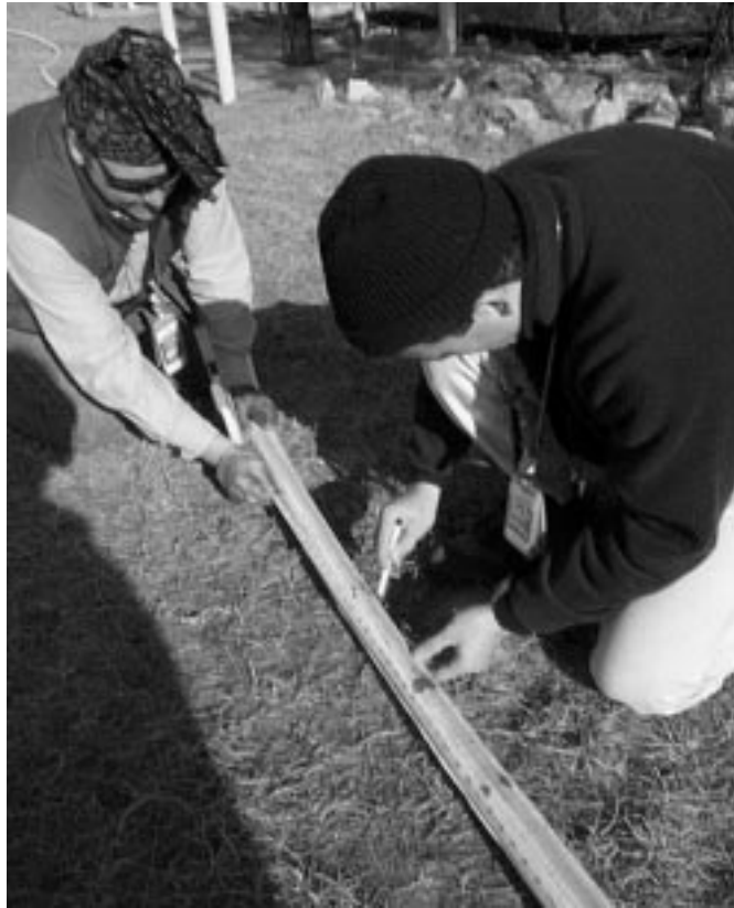
Figure 6. The membrane is turned inside out and examined for dyed spots.
