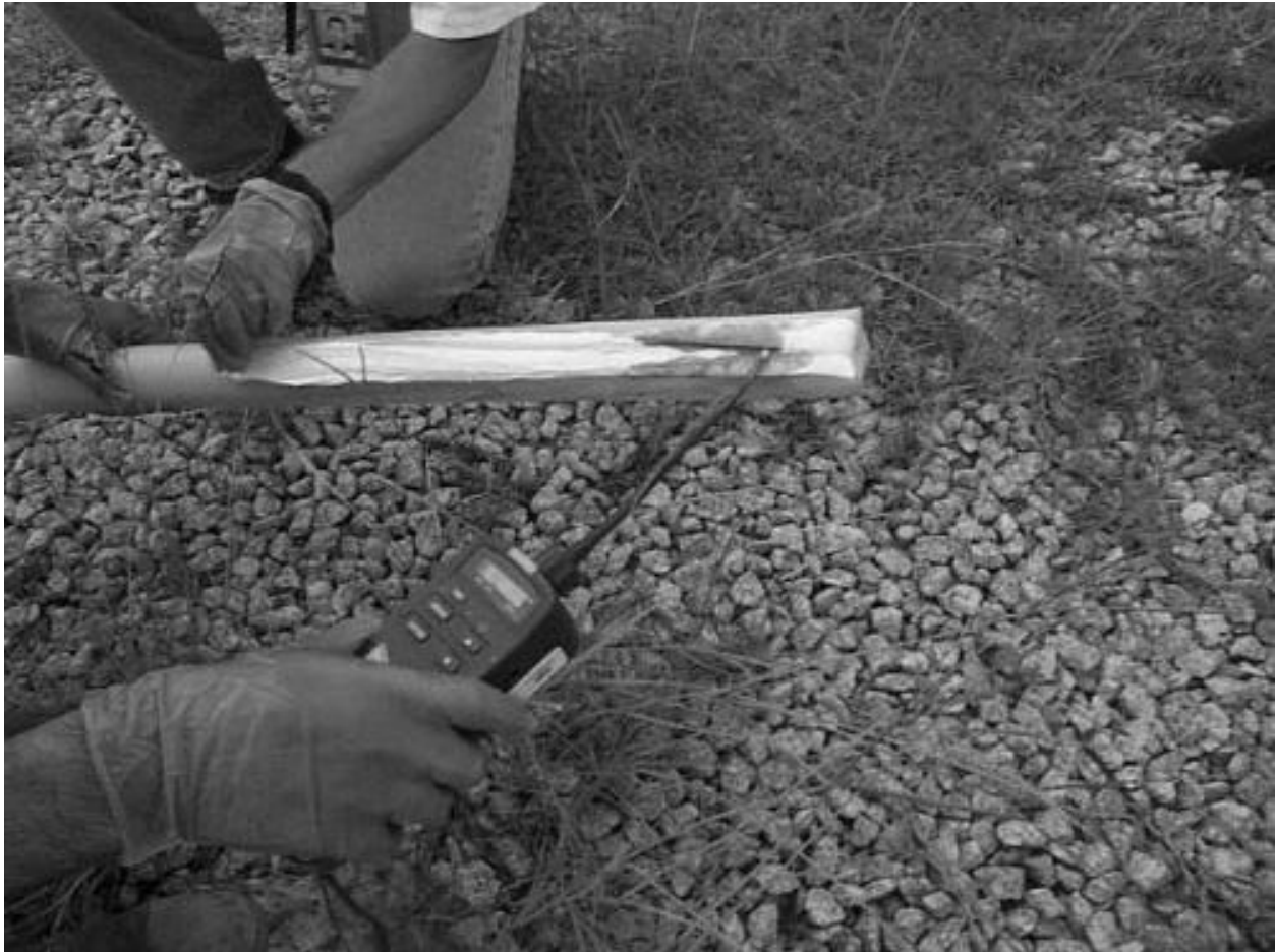
Figure 1. Section of Ribbon NAPL Sampler from 321-M
