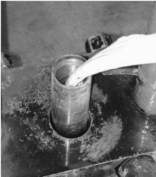
Figure 3. The bundled system is lowered into the CPT rods, the membrane is pressurized to break the seams, and the rods are pulled up.
