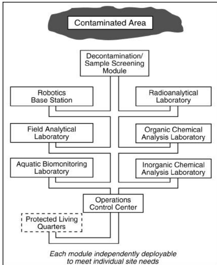
Figure 1. Schematic representation of the RTAL system.
