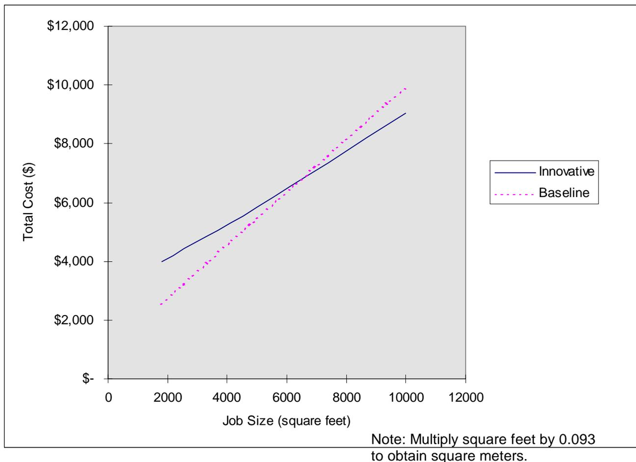
The extrapolation to 930 m<sup>2</sup> (10,000 ft<sup>2</sup>) assumes that there are six sets of anchor installations for the Wall Walker 2-D LMS and four repositions of the manlift for the baseline.
