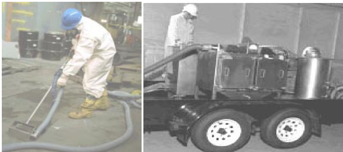
Figure 4. Photos of a steam vacuum cleaning technology.
