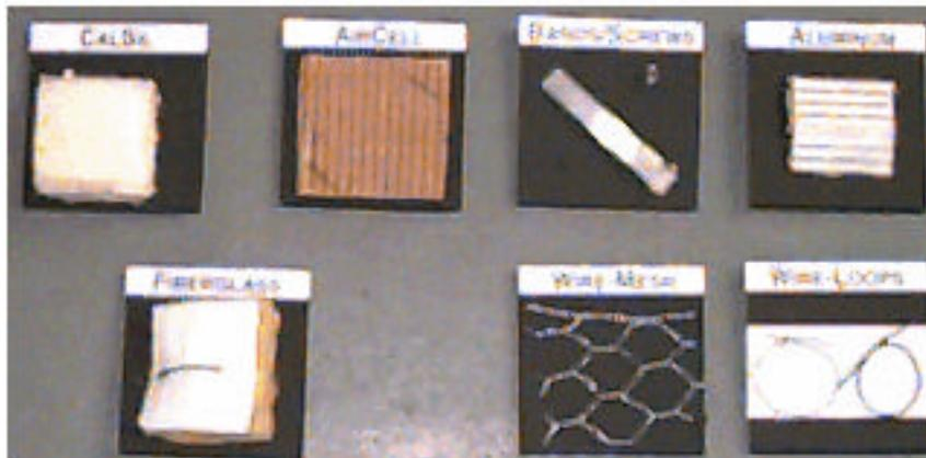
**Figure 6. Samples of lagging and insulation materials.**
