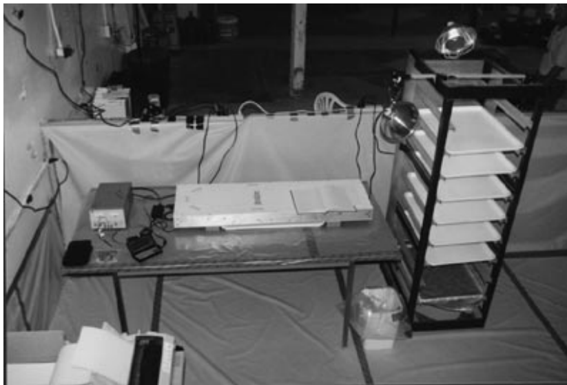
Figure 1A - At the LEHR site, samples were transferred to a nearby laboratory and placed in a standardized holder for rapid characterization. The surface/soil monitor can also be deployed in a dynamic conveyor configuration.
