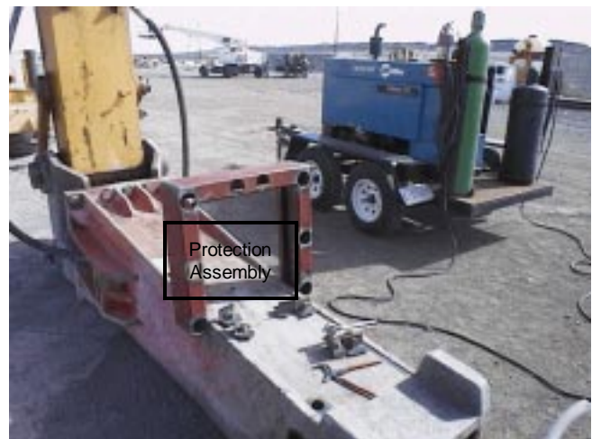
Figure 2. Protection assembly for spray manifold.
