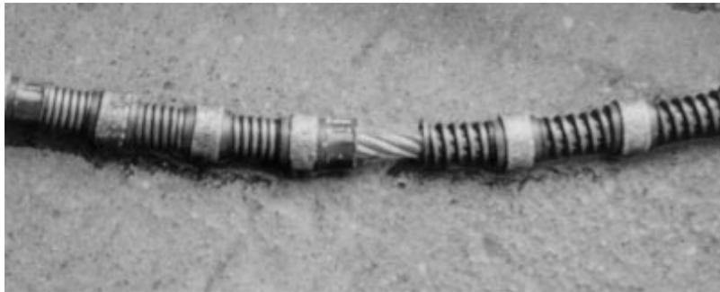
**Figure C-3. Damaged wire from Perma-Fill cut.**
