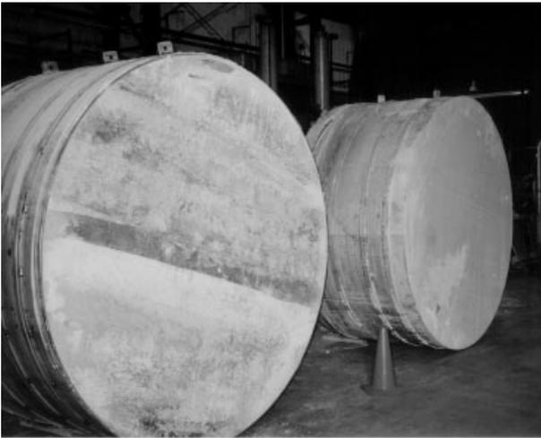
**Figure C-1. Rheocell – 15 and Mortar Void Filled Mockups..**
