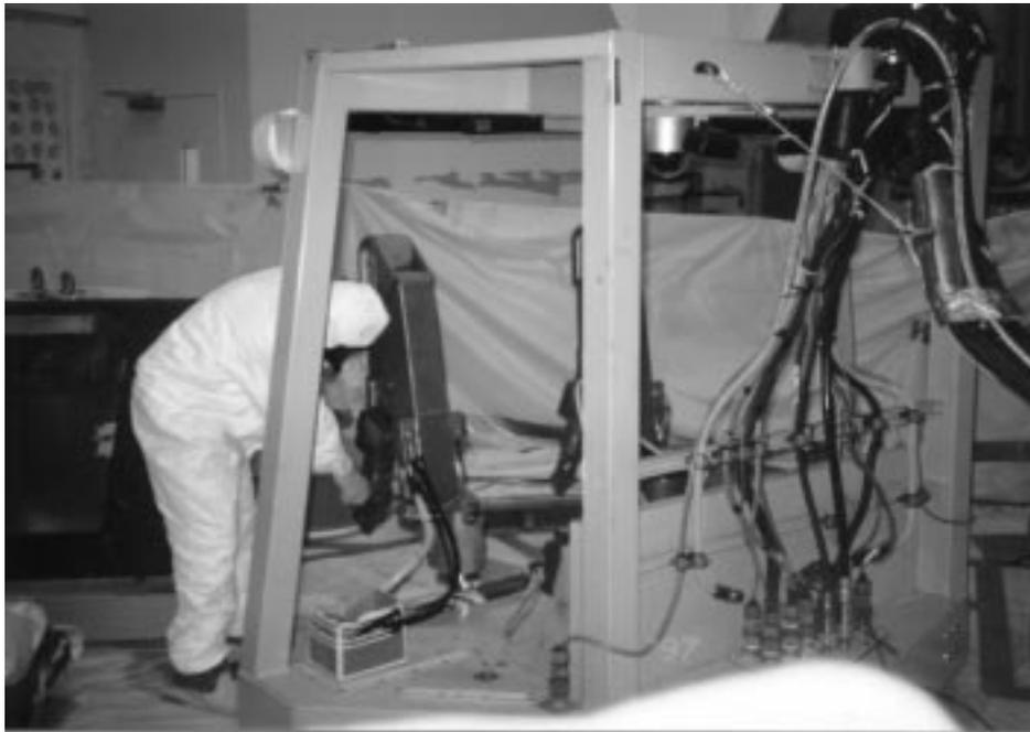
Figure 7. A Technician performs Maintenance on the DAWP
