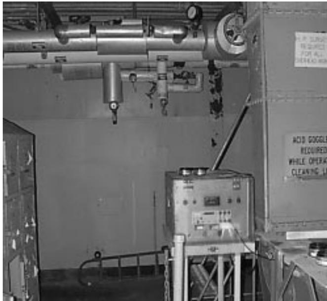
**Figure 3. Electret Ion Chambers placed in 321-M's Tube Cleaning Room**
