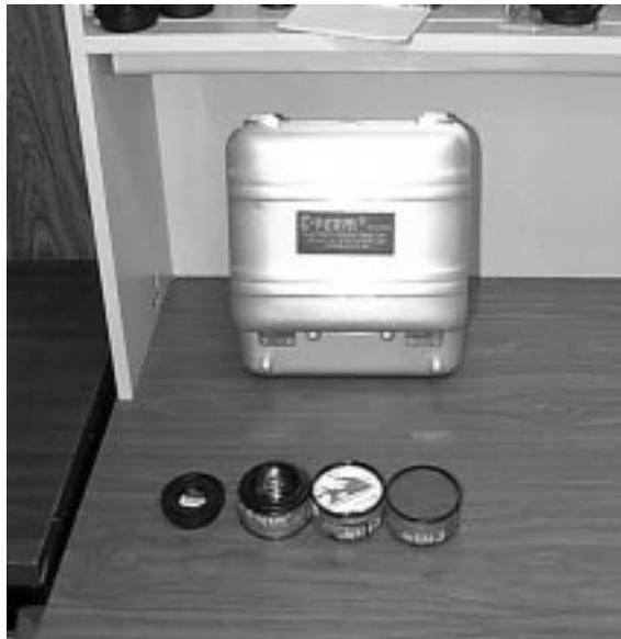
**Figure 2. SPER2 Microprocessor, electret, and 48 cm<sup>2</sup> ion chambers**
