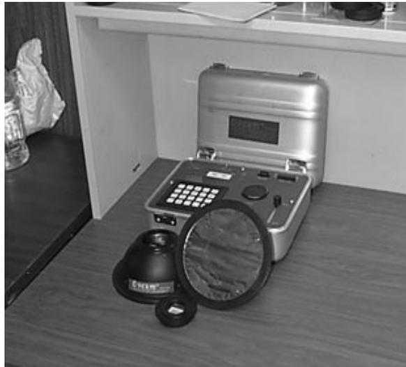
**Figure 1. SPER2 Microprocessor, electret, and 180 cm<sup>2</sup> ion chamber.**
