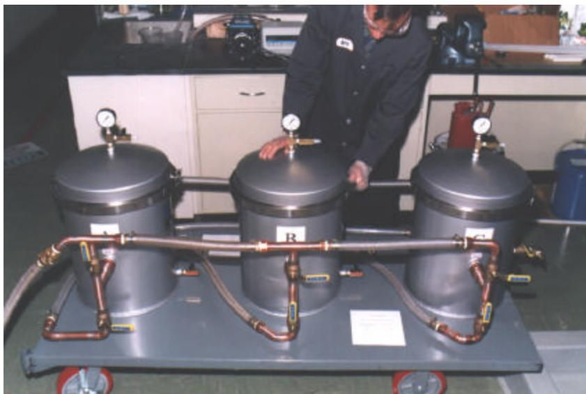
**Figure 2. Selective Separation Cartridges vessels in series.**
