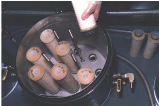
Figure 1. Selective Separation Cartridges in nested arrangement.
