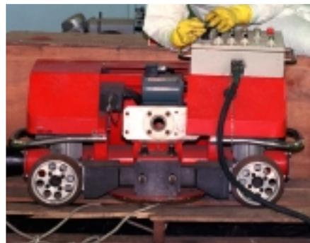
Figure 2. En-vac control unit with joystick sitting on top of the corner scabbler
