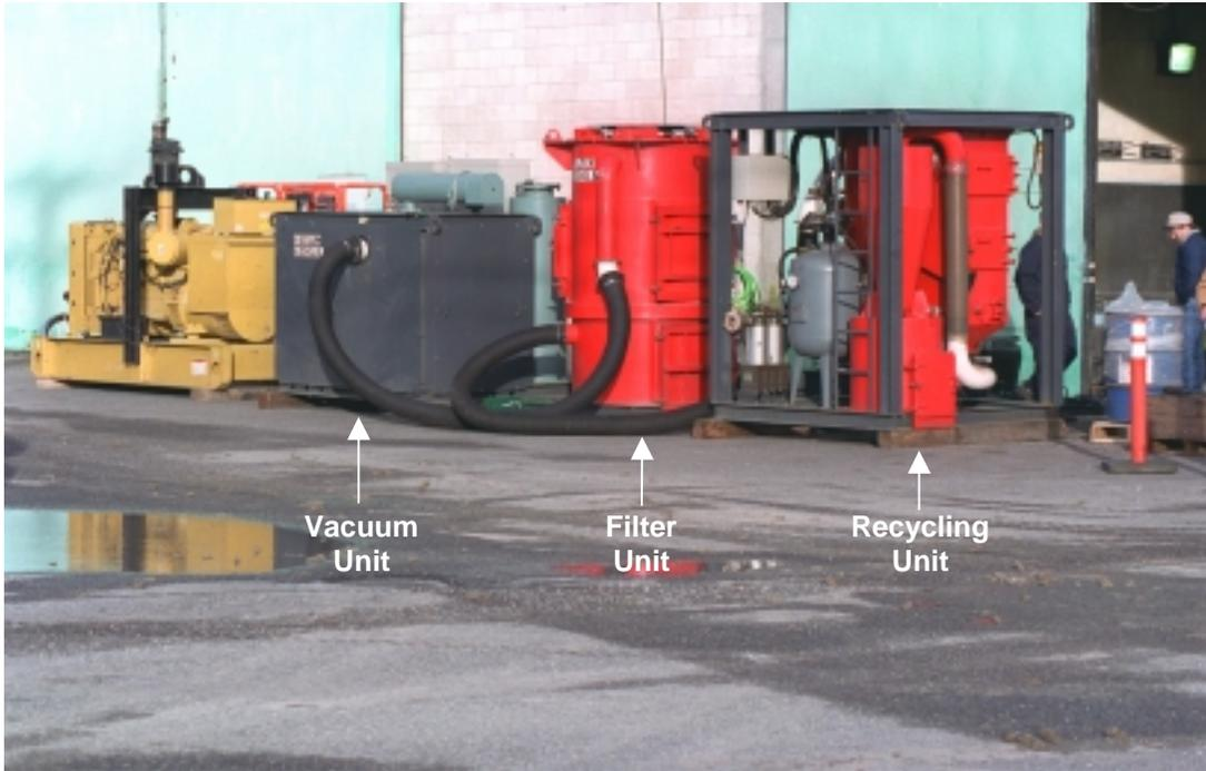
**Figure 3.** En-vac Blasting System
