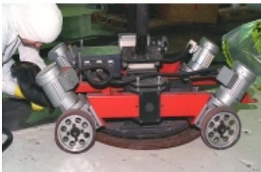
Figure 1. En-vac Robotic Wall Scabbler
