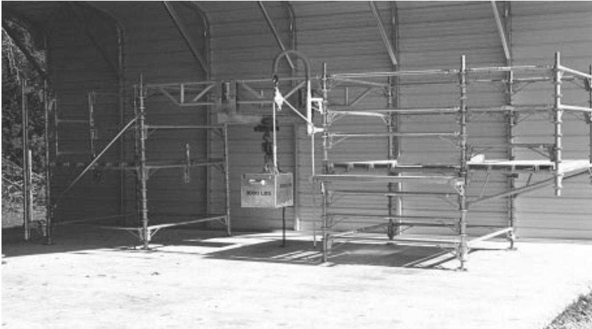
**Figure 9. Excel Scaffold with cantilever, lifting attachment, and truss attachments.**
