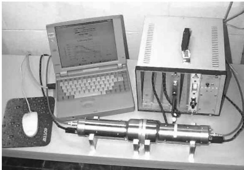
Figure 1. Field transportable beta spectrometer equipment..
