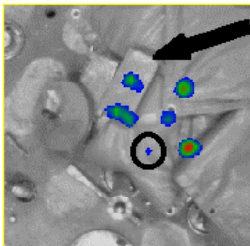
**Figure 8. Radiation field after placing lead brick.**
