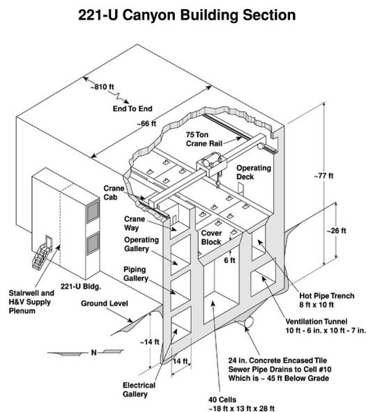
Figure 4 Cross Section of the 221-U facility.
