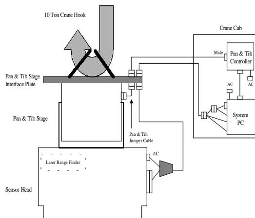
Figure 2 GammaModeler™ Setup
