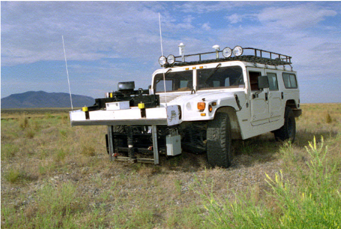
Figure 1. The Global Positioning Radiometric Scanner System used at the INEEL.
