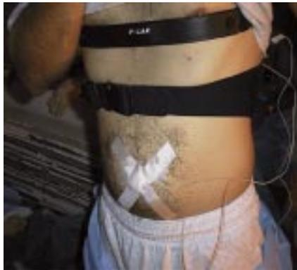
**Figure 3. Naval & skin temp. and heart rate probes as installed.**
