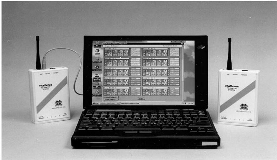
**Figure 1. Laptop PC and transceivers with probes attached.**
