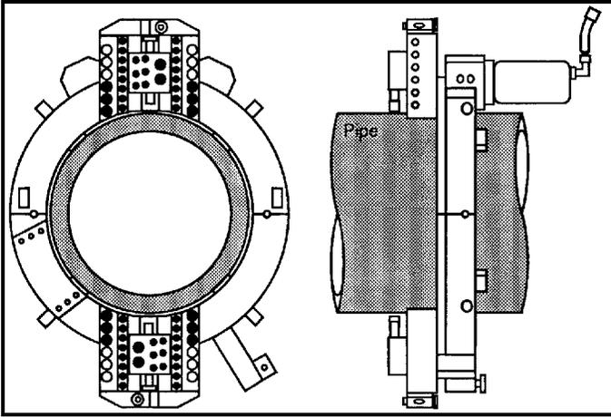
Figure 1. High-Speed Clamshell Pipe Cutter.
