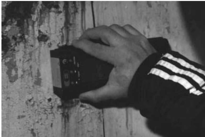
Figure 3. Niton 700 Series Multi-element Analyzer performing multi-element analysis on a wall.
