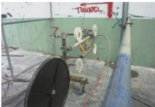
**Figure 2. Diamond wire saw.**
