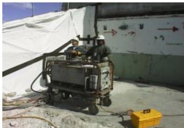
**Figure 3. Electric/hydraulic power unit.**
