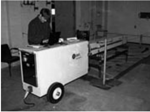
Figure 4. IonSens™ setup in RBA and CA Figure 5. Loading measurement chamber in CA.
