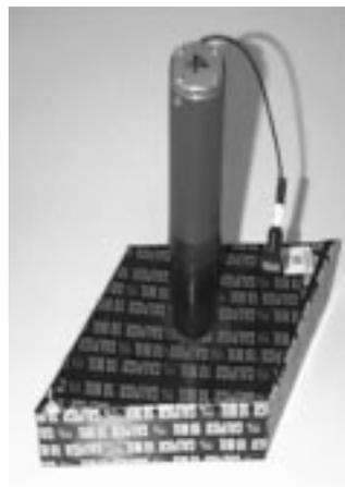
Figure 2 Individual scintillation detector used on MACS.
