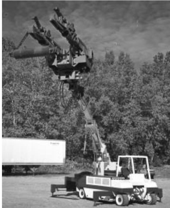
**Figure 9. MWP holding a 1,000-pound weight at the vendor's facility.**
