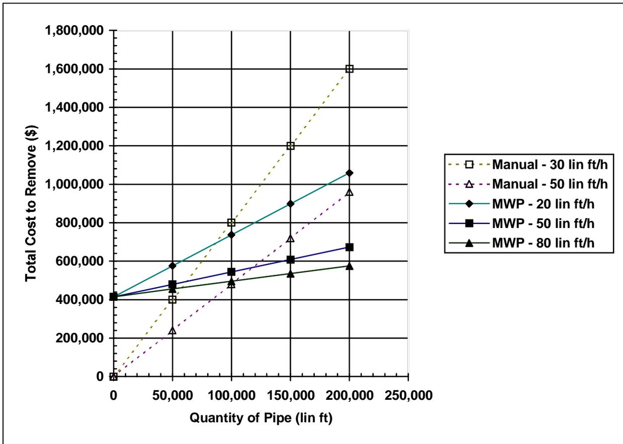
Figure 15. Total cost vs. quantity for various production rates.
