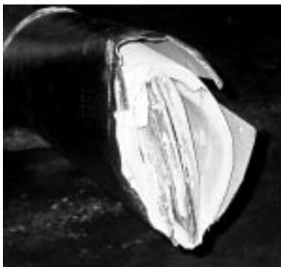
**Figure 10. 6 in, carbon steel pipe with insulation is crimped by the MWP.**
