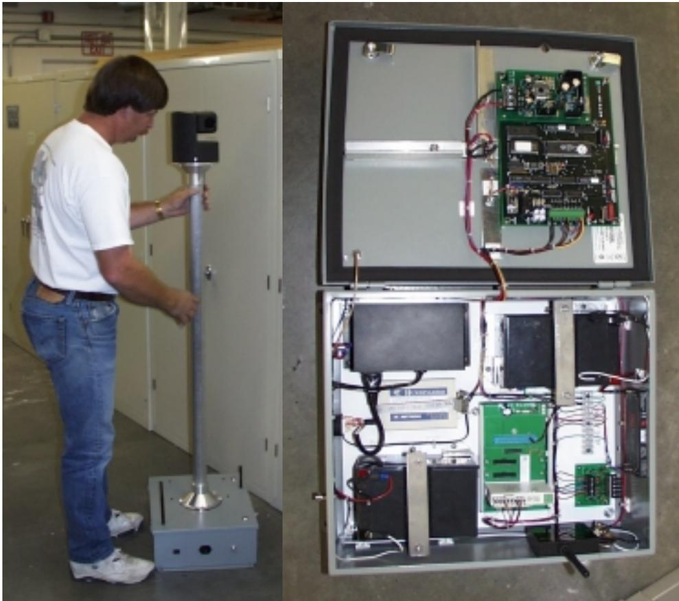
**Figure 5: The Facility Camera with its electronics enclosure.**
