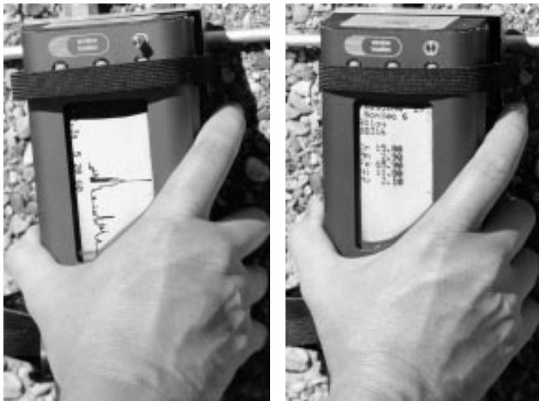
**Figure 1. NITON XL-800<sup>®</sup> Series Multi-Element Analyzer analyzing a small metal part using the irregular shaped part adapter. The image on the left shows the energy spectrum the instrument is reading during the analysis process. The image on the right shows the final element concentrations and alloy determination.**
