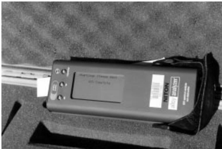
Figure 6. NITON® XL-800 Series Multi-Element Analyzer performing self-calibration
