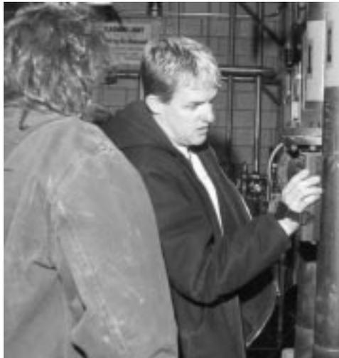
**Figure 2. NITON® XL-800 Series Multi-Element Analyzer being used to analyze system piping**
