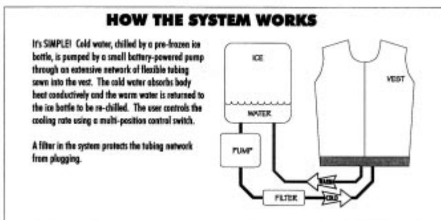
Figure 4. Schematic of the PICS.
