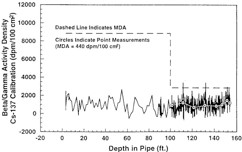
Figure 9. Survey results obtained during retrieval of the detector using the Cs-137 calibration factor.
