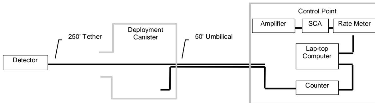
Figure 3. Block diagram of the measurement instrumentation
