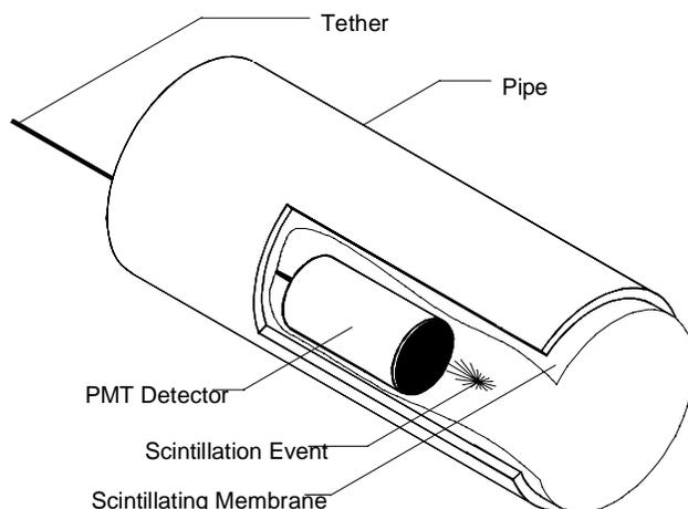
Figure 5. Sketch of Pipe Explorer™ Alpha Detector and Scintillating Membrane Deployed in a Pipe
