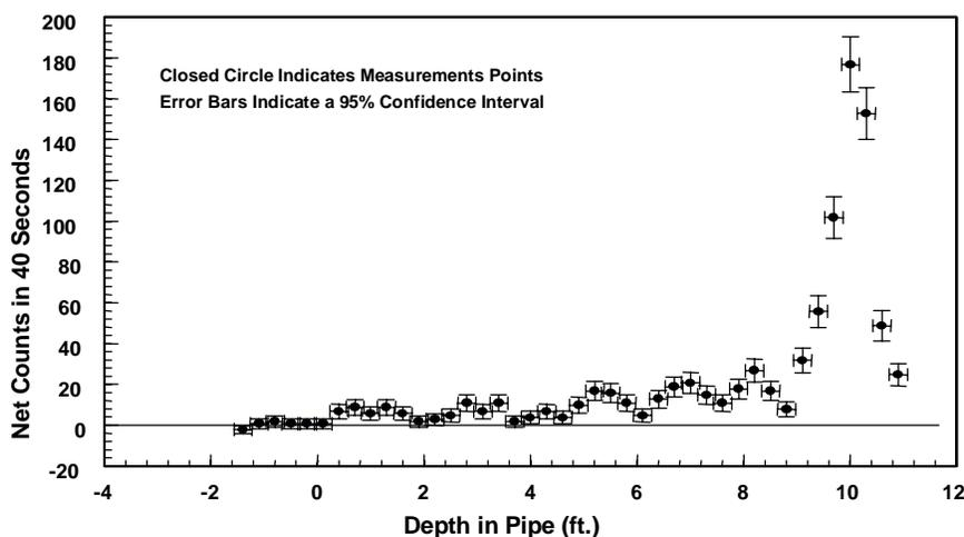
Figure 7. Results of Alpha Measurements in the CP-5 Fuel Rod Storage Tube #30
