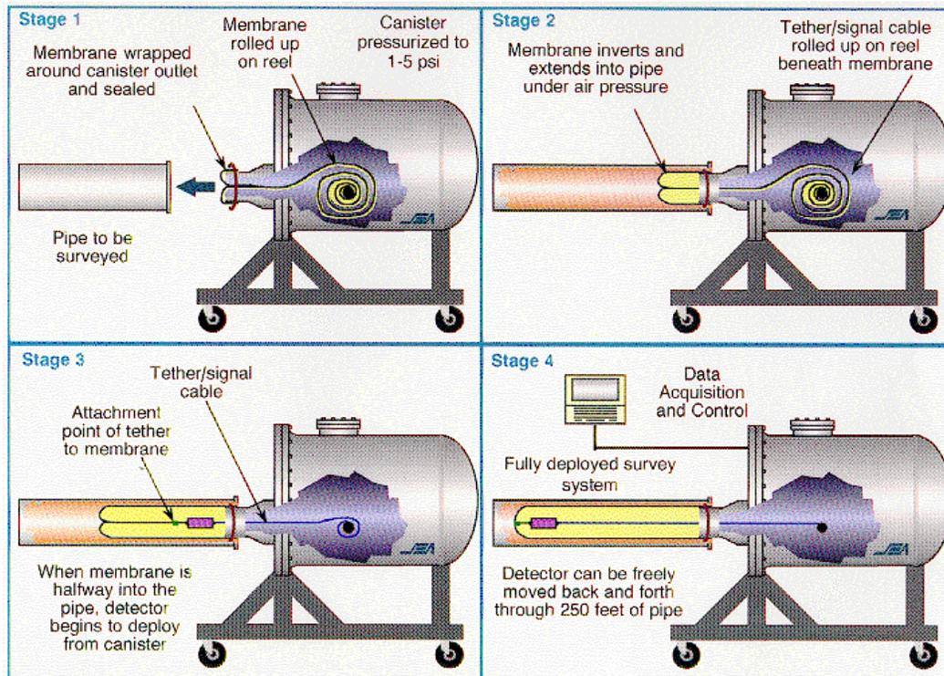
Figure 2. Deployment of the Pipe Explorer™ System
