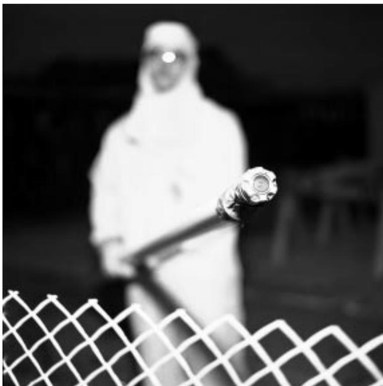
**Figure 1. The camera assembly on the end of the inspection probe.**
