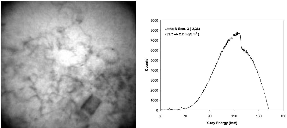
**Figure 14. Real-time X-ray image (12 cm x 12 cm) and associated K-edge spectrum obtained for one location on the ducts. The darker regions in the image correspond to the location of holdup material. The spectrum was acquired at a point near the center of the image.**
