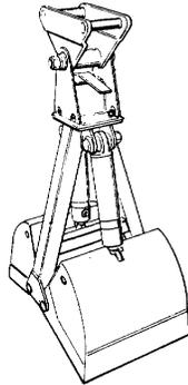
The Brokk 250 can be equipped with a 1/4 cubic yard clamshell bucket for difficult footing and interior excavating projects. The bucket can also be used for interior cleanup after a demolition job. The clamshell bucket is 18 inches wide, 4 feet long and weighs 400 pounds.
