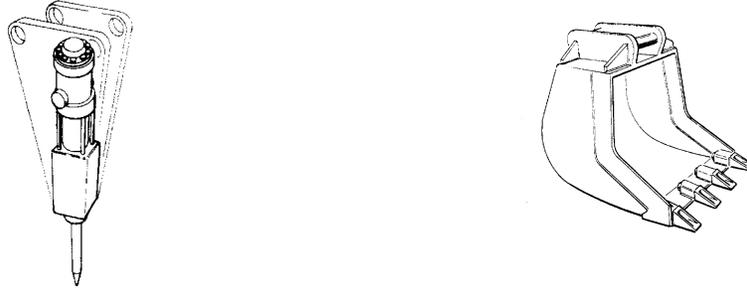
The Brokk 150 and 250 can both be equipped with excavating buckets. The buckets are available in various widths and can be supplied with either smooth cutting edges or toothed. The smooth edge bucket worked very well for interior clean-up and loading of debris. The toothed bucket is generally for excavating soil.
