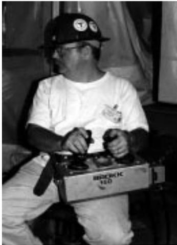
**Figure 2. Brokk remote controller.**
