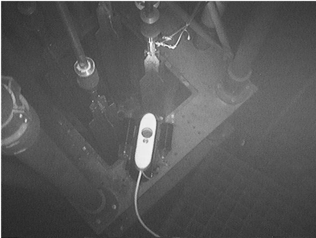
Figure 6. The RUCS vehicle characterizing a control rod
