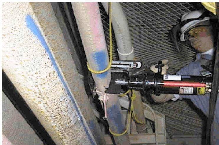
Figure 6. Baseline hydraulic shear.
