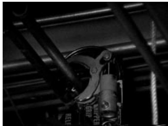
**Figure 9. Gripper mounted to shear head**
