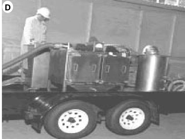
**Figure 2: Photos of the Kelly Decontamination SVC System. Photo C shows a worker demonstrating the 10-inch swivel steam/vacuum tool for cleaning floors and large surfaces. Photo D shows a worker operating the Main Control Unit. In front is the Demister/HEPA Filter Unit, and to the right is the Vacuum Unit. All three units were mounted on a trailer outside Building 1A.**
